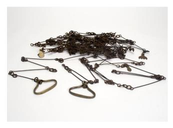
Old surveys were often measured using a Surveyors Chain. These were literally made up of 100 links. Each **CHAIN** was 66 feet long. Each link was 0.666 of a measured in chains (abbreviate Ch) simply multiply the distance in chains by 66.
